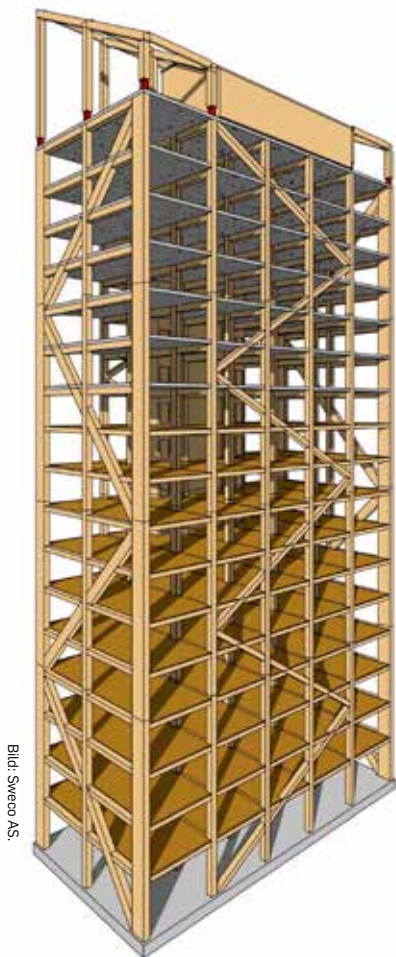
Figur 4. Mjösatornets bärande system.
